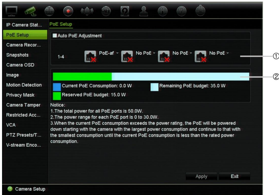
Figure 23: PoE power budget information on IP cameras (4-channel PoE recorder shown)
