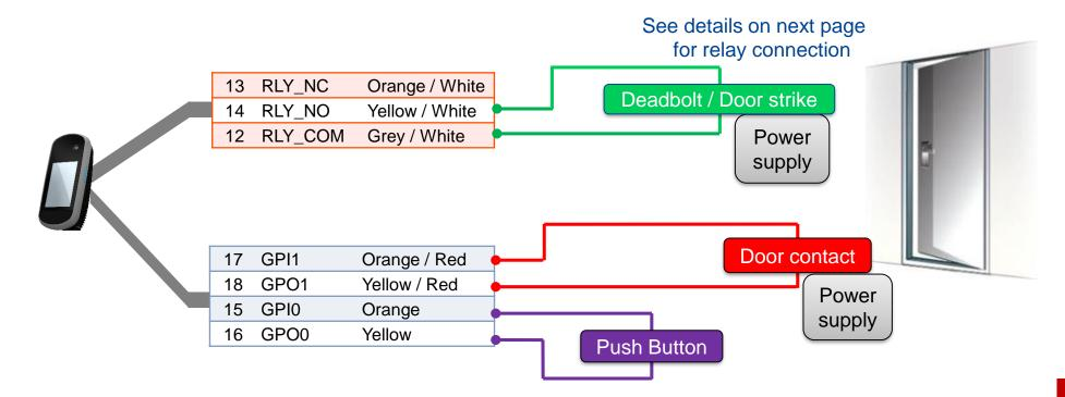
If door contact is not used, GPI1 (17) and GPO1 (18) shall be connected together
