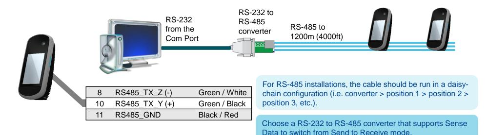
Use CAT-5 UTP (or better) cable (shielded recommended) with a characteristic impedance of 120 ohms.
