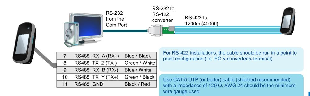
Choose one twisted pair of conductors to use for RS485\_TX\_Y (TX+, Green / Black wire - 10) and RS485\_TX\_Z (TX-, Green / White wire - 8).
