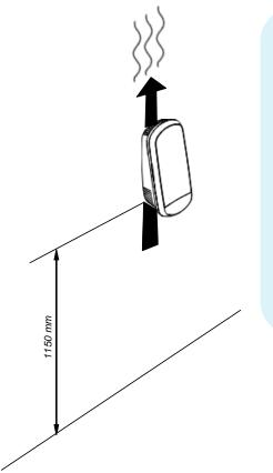
If several devices are installed in parallel lanes (typically for gates or turnstiles), then a minimum distance of 80cm must be kept between the devices.
