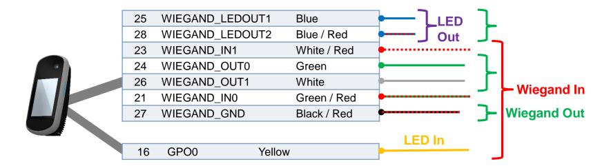
Three-conductor cable (shielded recommended) is required for Data 0, Data 1, and WGND.
