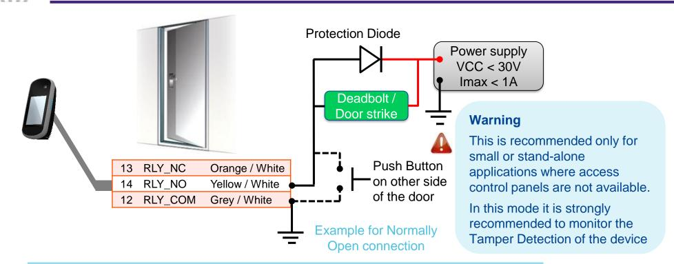
Inductive load management requires a parallel diode for a better contact lifetime.
