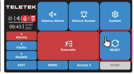
The panel is reset to Normal operation mode.
