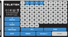
In case of Operation in Network, choose the panels, where to perform Turn off Buzzer.
