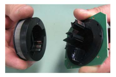
5. First you have to clean the internal part and then the external part of the chamber. Afterwards clean the PCB as well.]
