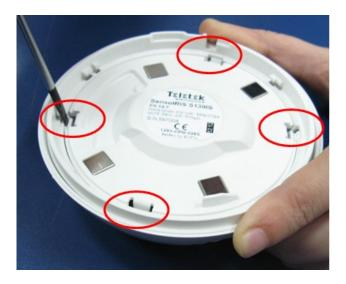
2. Next you have to remove the PCB from the base. That is done by pulling out the plastic trotter and slightly pulling the PCB up.
