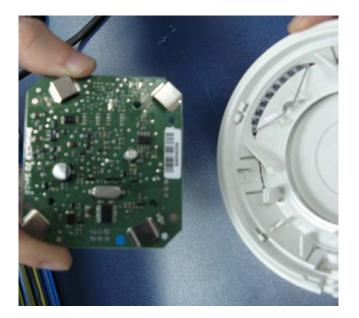
3. The removed PCB has to be disassembled with a screwdriver. BE CAREFUL WITH THE PLASTIC SIDE HOLDERS.
