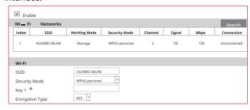
Check 'Enable" to enable Wi-Fi. Then click 'Search" to refresh the wireless device list. Select the desired router, enter the key number and select encryption type. After that, select 'Obtain an IP address automatically" or manually enter the IP address by clicking 'Use the following IP address". Then click 'Save" to save the settings.
