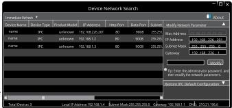
3 Double-click the camera listed in the IP-Tool to connect IP camera. The default IP address of this camera is **192.168.226.201**.
