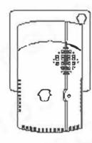
Do not mount the detector to the gas over lest it should suffer reacting from fife; do not mount it in position with much lampblack to avoid faire alarm or air later touvers dogged which might effect the terrativity of defector; do not mount it near to exhaust fair, door or window, butteroom, and other places with much water vepor.
