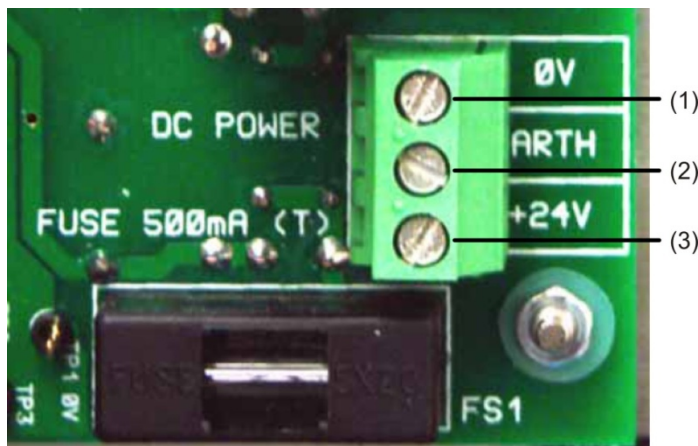
Figure 19: Command module power supply connections
