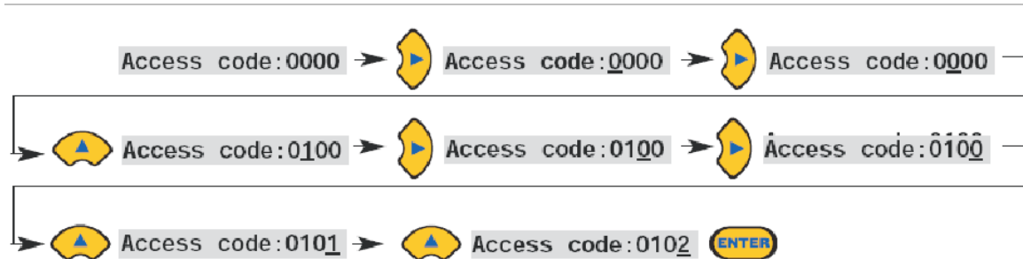
Figure 27: Setting the access code
